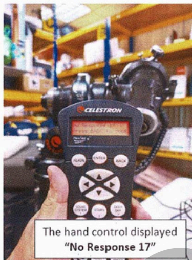
The DEC motor port/connector is damaged
